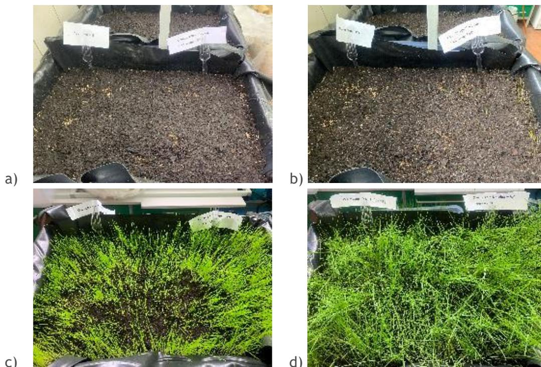
**Fig. 8.** Pictures from experimental cultivation of grass on the ground containing soil and woollen nonwovens from wool waste - made in ATH (on the left side of each photo) or rope containing in the outer covering woollen nonwovens from wool waste and a core of wool dust (on the right side each photo): a) on the day of sowing, b) 6 days after sowing, c) 10 days after sowing, d) 22 days after sowing.
