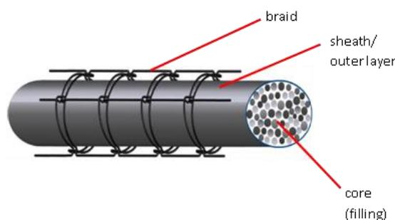
**Fig. 6.** Scheme - structure of cord/rope
