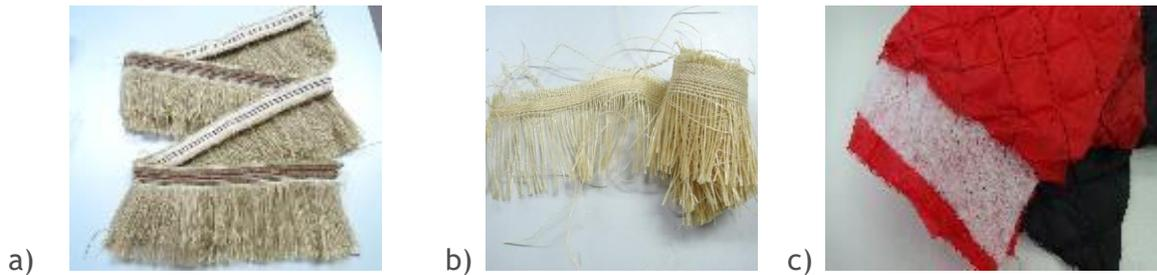
**Fig. 3.** Post-production waste used for the production of nonwovens: a) jute selvages, b) polypropylene selvages, c) quilted cuttings - polyester
