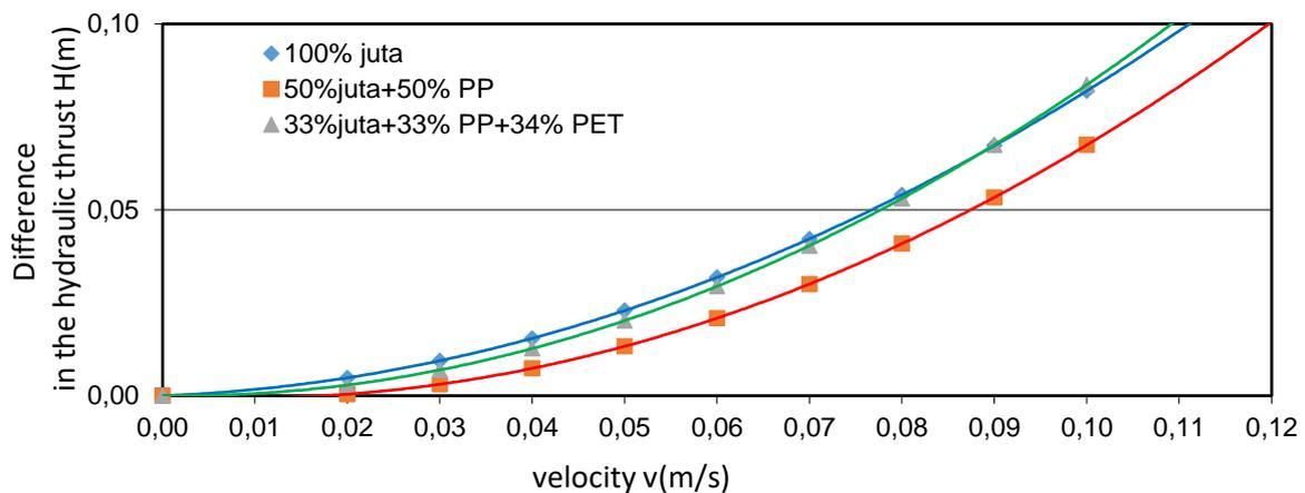
*Fig. 5. Diagrams of water permeability perpendicular to the surface of the geotextile without load for needled nonwovens made of defibred post-production waste*
